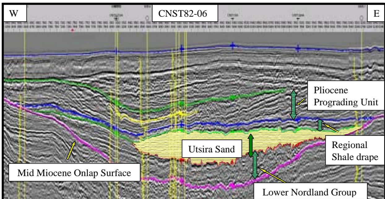
Fig. 1. West-east seismic section (CNST82-06) and well-cross-section through the Utsira Sand and the Pliocene prograding system in the Sleipner area. Location is indicated in Fig. 2.
