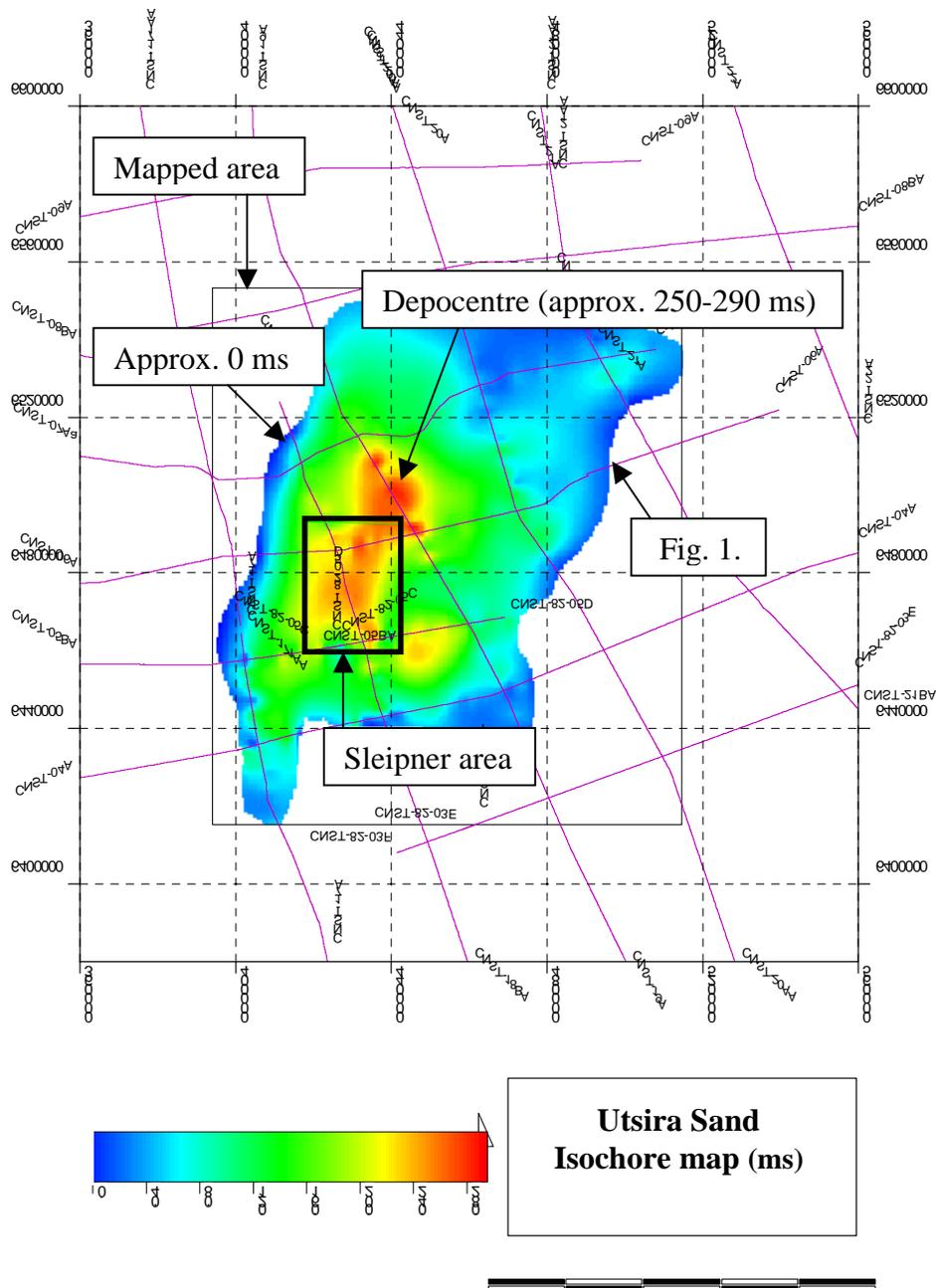
Fig. 2. Two-way time isochore map (milliseconds) of the Utsira Sand. The Sleipner area (site for the CO<sub>2</sub> injection) is located within the depocentre. Location of Fig. 1 is also indicated.
